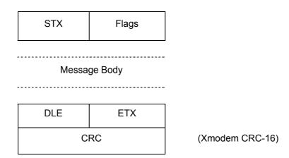
Transmission order is from top left (STX) to bottom right (second byte of CRC). The STX, DLE and ETX fields refer to the eight-bit ASCII control codes with those names, their byte values being 0x02, 0x10 an 0x03 respectively. CRC is a 16-bit *Cyclic Redundancy Check* field, a description of which appears below. A table driven algorithm for calculating this type of CRC is given in appendix A.
